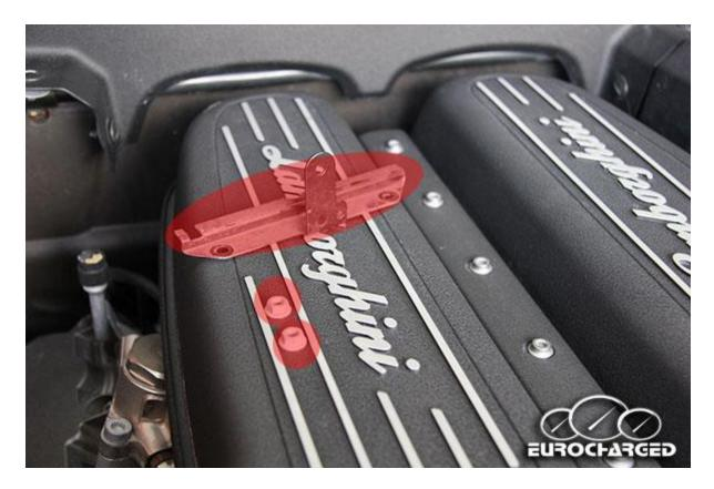
Remove the nuts and metal support for the ecu.
