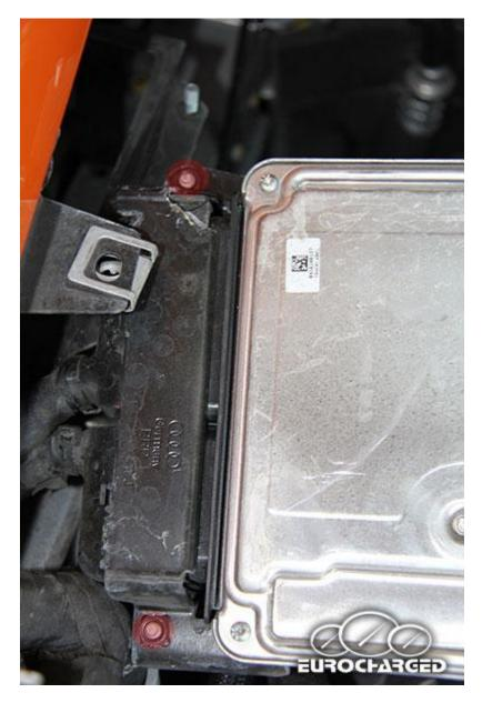
Remove the bolts that hold the ecu harness. You should then be able to pull the tab to release the ecu from the harness. As indicated before, please make sure to mark the driver's side ECU when shipping them in.
