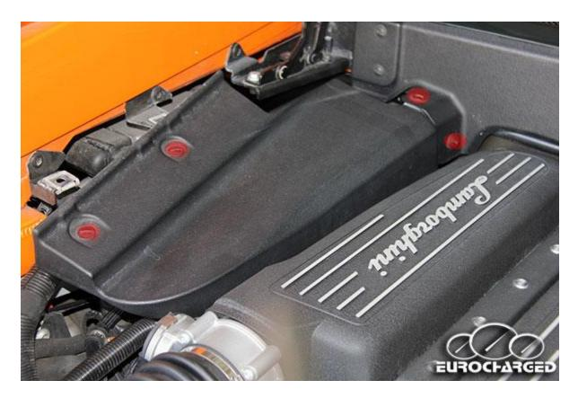
Now look at the engine. Highlighted in red you will see screws that need to be turned in order to get the cover off. Take a flathead screwdriver and unscrew the cover. The screws will not come out, but simply will release the plastic cover.
