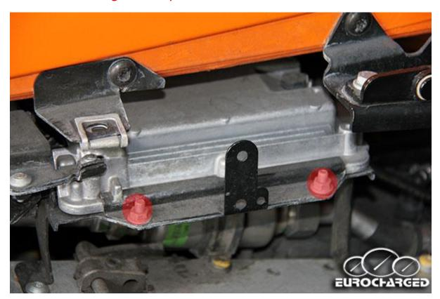
Using a 10mm socket, remove the screws that are highlighted in red.
