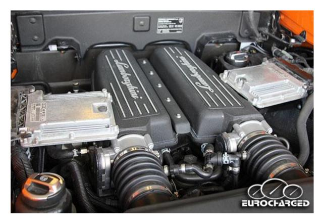
There are two ecus in the car, one on the driver's side, and one on the passenger side.
