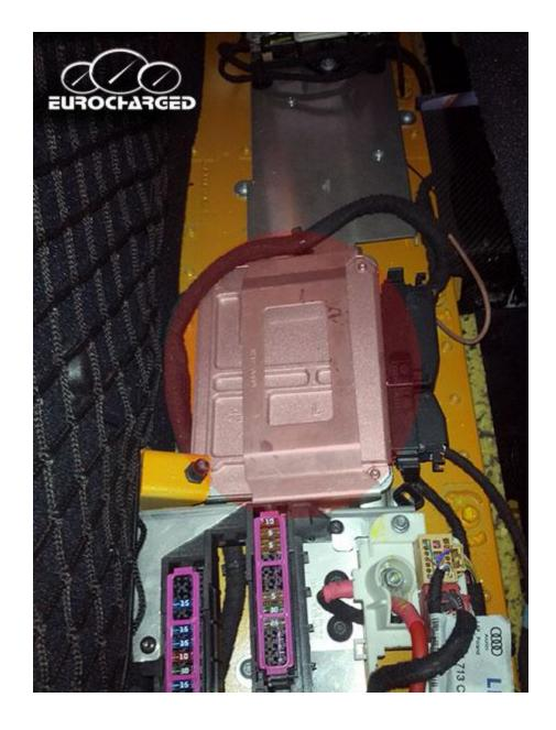
Remove the shelf and you will be looking at the fuse box as well as the TCU module. The TCU is located on the left side if facing the engine. Remove the tcu hardness by pulling the tabs to the right and left. The TCU itself is held on by 10mm bolts. Remove them and you should be able to remove the TCU.
