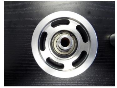
3. Insert new bushing onto sleeve against bearing of 6 rib pulley.
