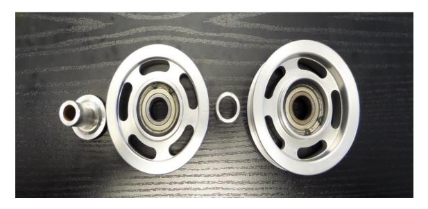
2. Insert sleeve from old idler assembly into 6 rib pulley; be sure the snap ring faces up.
