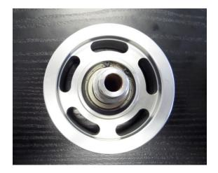
4. Take the 8 rib pulley and make sure the snap ring side goes toward bushing and 6 rib pulley.
