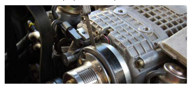
Step 9- Reverse installation. Run the belt through the upper idler before bolting it on. Torque the upper idler bolt to 20nm. The remaining bolts can be hand tightened.
