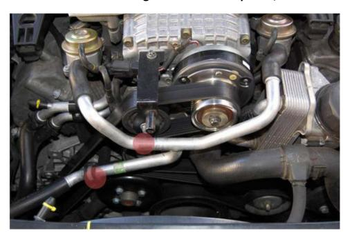
**Step 2-** Using the E11 torx, loosen the belt by turning the tensioner counter clockwise. Slip the belt off the middle idler.
