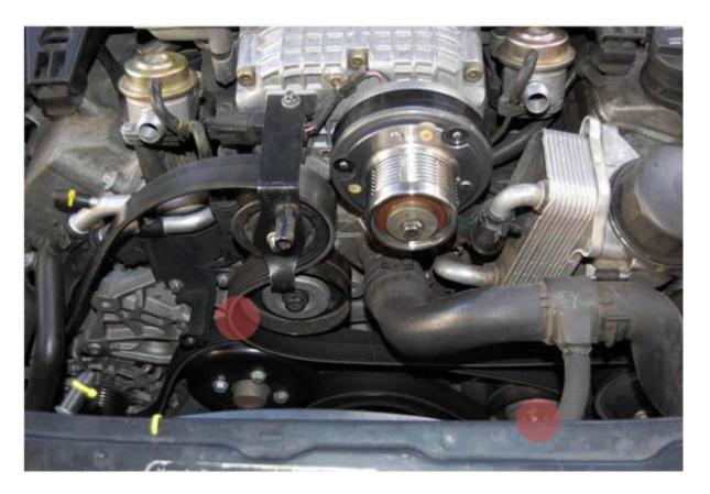
**Step 3-** Remove the upper idler pulley. The bracket bolt is a E10 torx. The pulley is a E12 torx. Remove both the pulley and bracket
