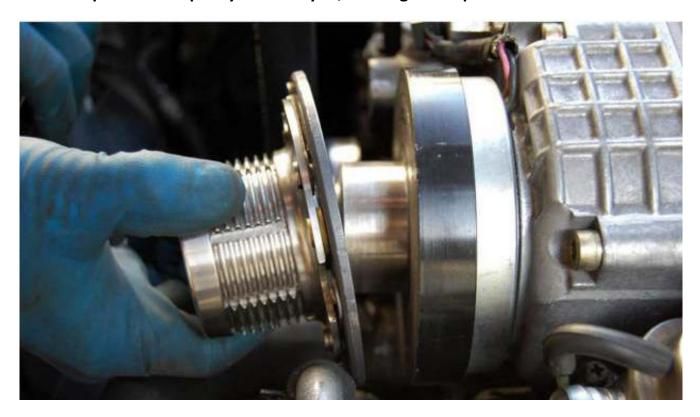
Step 7- Place the new pulley on the shaft, and replace the stock washer and bolt. Tighten them down using the previous method of holding the clutch. Check the gap between the back plate and the clutch. It should be between .20-.30 mm. The important point is that once tightened, the pulley and clutch spin freely of each other, while being as close as possible. If you need shims for you pulley contact us and we can provide them to you.
