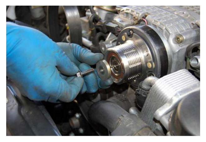
Step 6- Pull the pulley towards you, and angle it as pictured to remove it.
