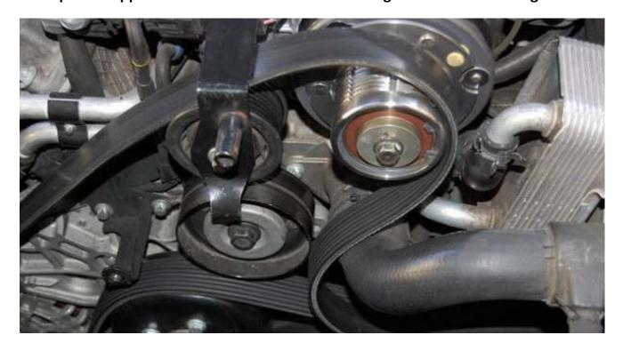
Step 9- Go over each bolt and ensure it was tightened properly. Turn the SC Clutch by hand, and it should spin freely. Check the belt for proper alignment on the pulleys. Once everything has been verified, start up the car. Observe the belt and pulleys, making sure there is no awkward wobbling or noise. If all look well, go have some run on the road.
