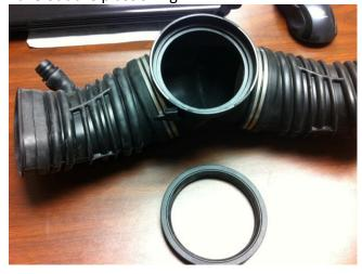
2. Remove the rubber O ring attached. You will not use the plastic part
