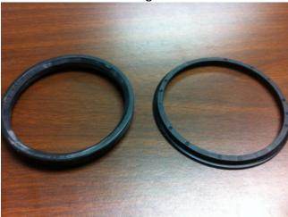
3. Flip the rubber O ring and put that on the TB.
