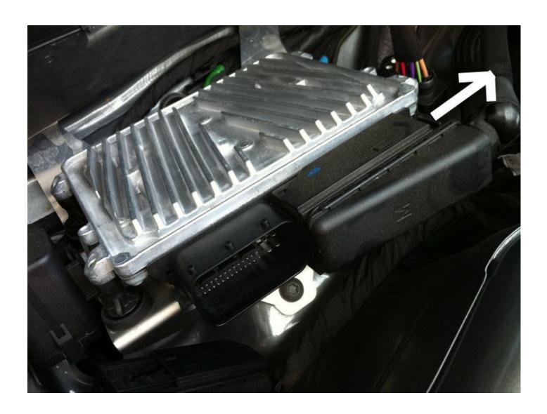
Once this is done, all you need to do is pull out the ECU. It is not held in place by screws but rather slipped into 4 rubber mounts (1 on each corner):
