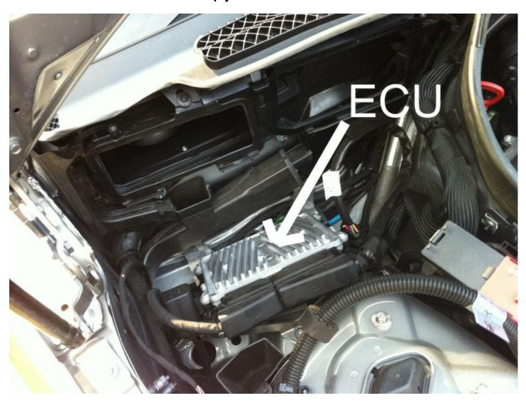
Then you need to pull out the 2 connectors. On the outside of each of these connectors is a big sideways T shaped PULL TAB. Just pull it out gently about 1-2 inches) and this will safely unlock AND pull out the connector:
