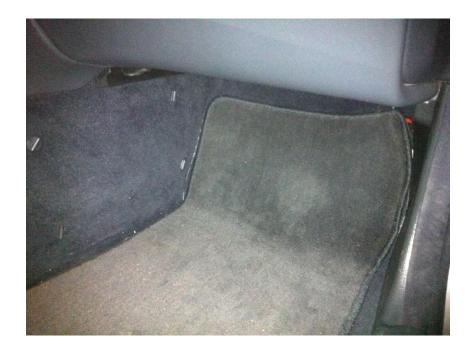
Pull the carpet and foam padding back from the passenger floorboard, up near the console. You will need a 10mm socket wrench with an extension. There are three bolts that hold the metal plate in place.
