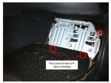
Once the bolts are removed, pull the plate back and up. The TCU is located on the back of the plate. You will need an 8mm socket to remove the two bolts holding the TCU in place. Then pull the two connectors out of the TCU.
