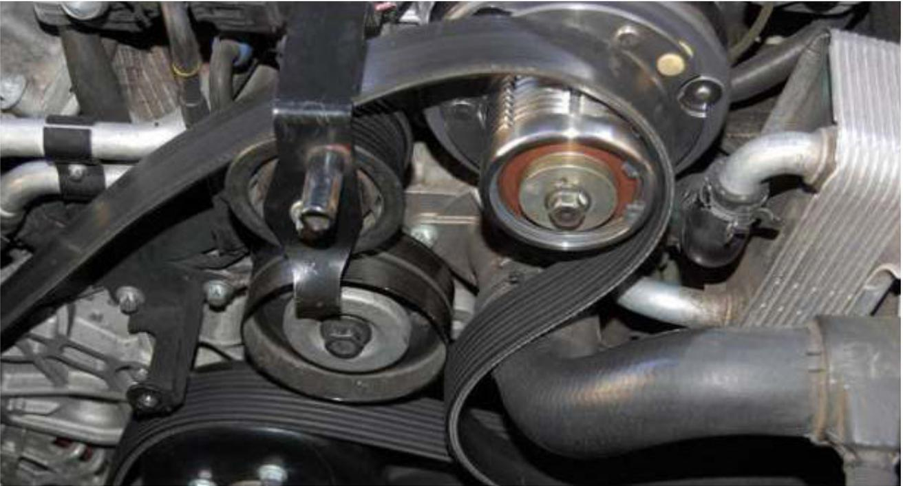
**Step 9- Go over each bolt and ensure it was tightened properly. Turn the SC Clutch by hand, and it should spin freely. Check the belt for proper alignment on the pulleys. Once everything has been verified, start up the car. Observe the belt and pulleys, making sure there is no awkward wobbling or noise. If all look well, go have some run on the road.**
