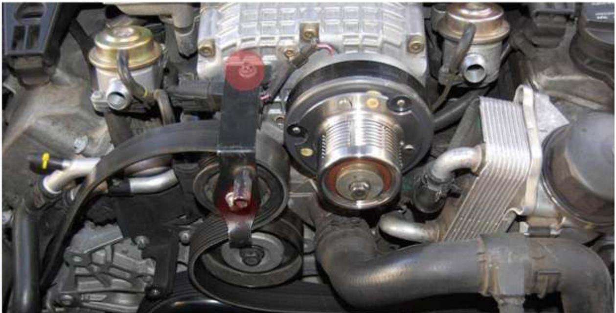
**Step 4-** Place a mat or piece of rubber pad under the SC clutch. Using the upper idler standoff as a fulcrum, place the large screwdriver or crowbar under the pad, and apply light pressure to keep the clutch from spinning. While holding it, use the 12mm socket to loosen the sc pulley bolt. You can also use a strap wrench to hold the pulley while removing the bolt. (simple method)
