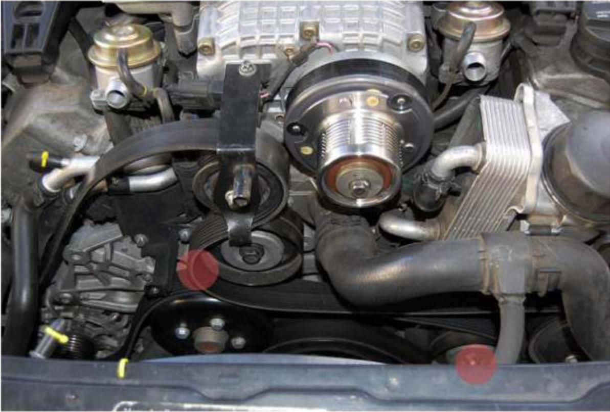
**Step 3-** Remove the upper idler pulley. The bracket bolt is a E10 torx. The pulley is a E12 torx. Remove both the pulley and bracket
