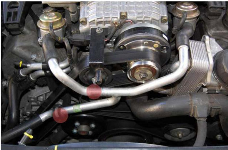
**Step 2**- Using the E11 torx, loosen the belt by turning the tensioner counter clockwise. Slip the belt off the middle idler.
