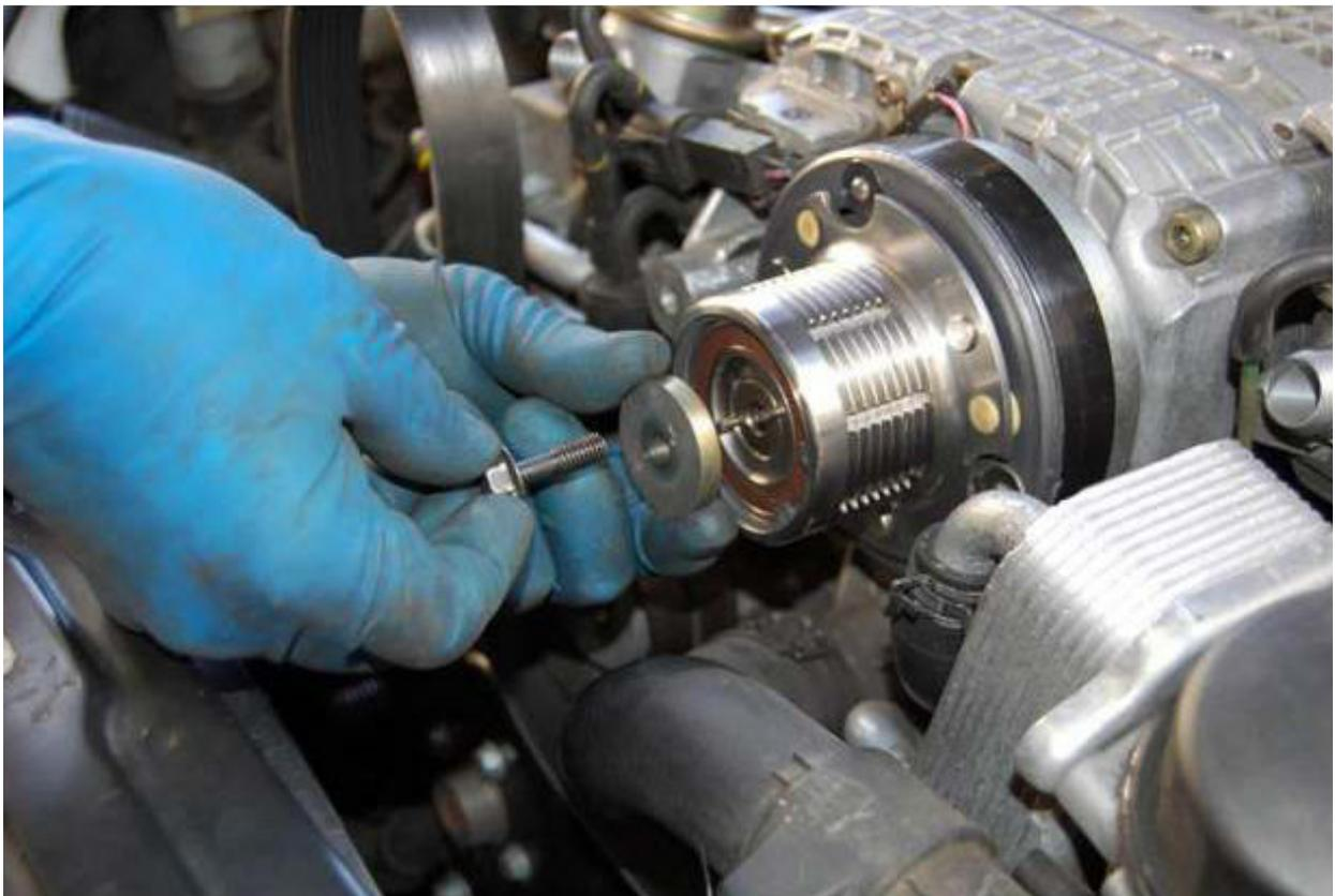
**Step 6- Pull the pulley towards you, and angle it as pictured to remove it.**
